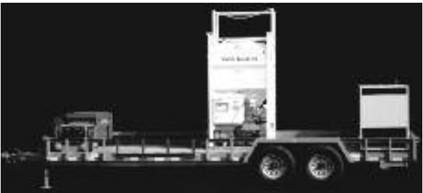
StoSilo Mobile Includes the StoSilo Combo, air compressor, water pump and generator mounted on a truck with one ton (907 kg) of towing capacity TO "3/4 ton or larger truck with a Class III towing package equipped with electric brakes; a 2-15/16" ball is required.
