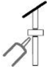
4. Sealant at penetrations
